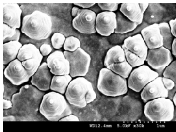
Fig 1: This HR-SEM is a magnification (scale bar = 1 μm) of hexagonal nanopyramids. This was grown under an equal mix of Ar/O 2 . As the particles land on the surface, there is a lower potential for the particle to nucleate a growth site at the flat regions (i.e., near the centre) or next to an edge rather than to locate itself on top of an edge. This is due to a greater attraction due to surface potential. This process continues until this terraced pyramid shape forms.
