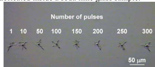
Figure 3: Voxels in soda lime glass.
